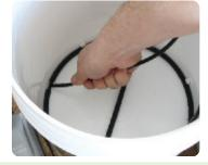
Attach the ends of the air supply lines to the T-connectors on the diffuser ring.
