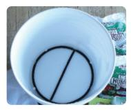
Remove all contents from the brewer. Do not disturb the diffuser ring at the bottom.
