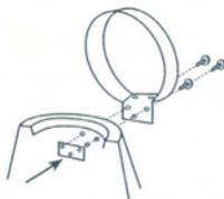
**STEP 4.** Place the green outer cone over the black inner cone; making sure that the lid opens in a convenient direction. Line up the screw holes in the base of the green outer cone with the notches on the base of the black inner cone. Use six 10x5/8 self-tapping screws to secure the cones to the basket.
