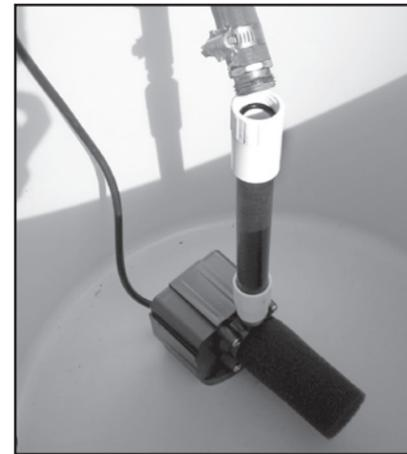
Connect hose to Swivel Fitting to drain.
