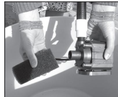
Remove Filter from Pump to clean.
