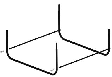
**C.** With lower support sections held upright, as above, fasten the other support spacer in a similar manner with 2 additional 1/2" bolts to form the assembly shown in the adjacent photograph.
