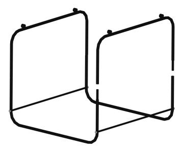
**B.** Slip the ends of the upper support fully into and over the uprights of the lower support section. Repeat with the second support. *Continued...*
