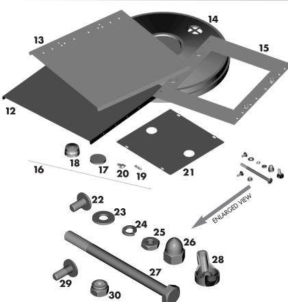
**Note:** The Tie Rods (Item 16) have been shipped inside the Support Spacers (item 2). Be sure to remove them before assembling the frame.
